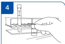
Immediately recap the vial with the hydrated material and place into a 34°C-38°C incubator for 30 minutes to ensure complete hydration.
